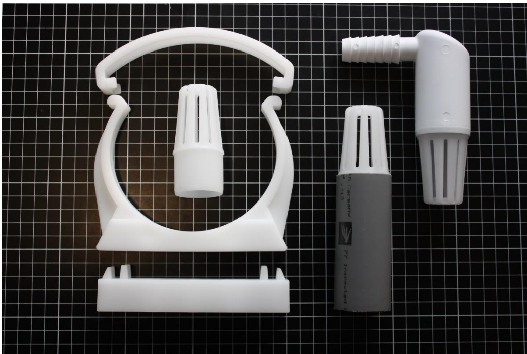
Abb. 1 / mounting bracket for wall or floor mounting (DN 120), with clamp und adapter for installation height. Pipe sieve (DN 40) with HT pipe length 90 mm and angle nozzle DN 40 /20.
