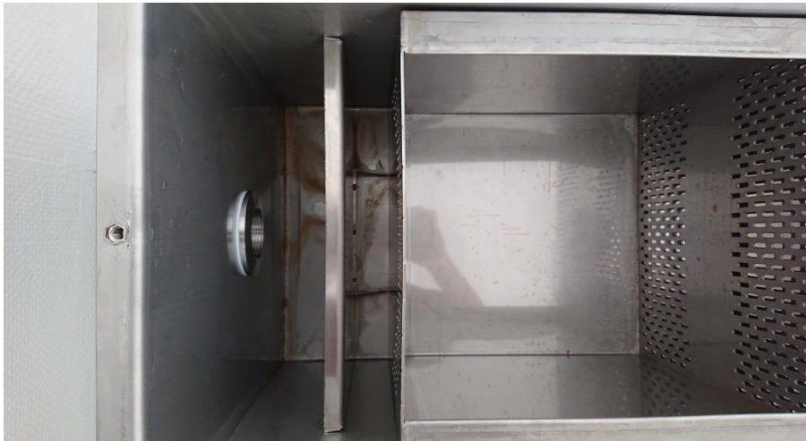
Condensate outlet pipe with basket locking function
