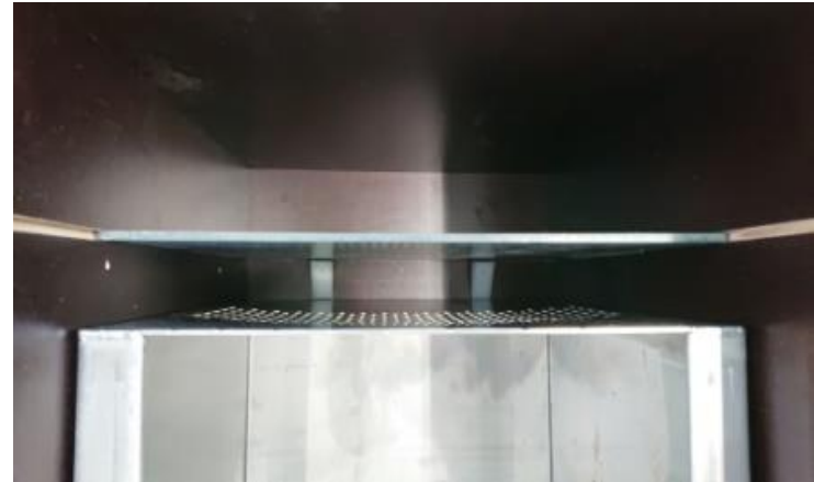
Prototype with neutralising basket locking function (above)
