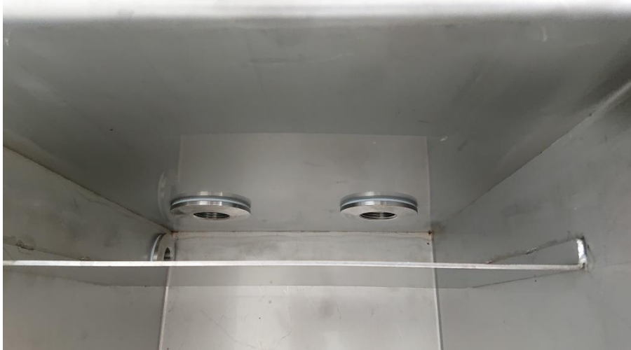
Condensate outlet pipe with basket locking function
