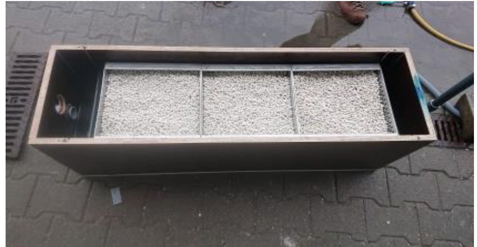
Step 3 – Checking of water flow behaviour with neutralising agent
