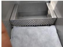
Mount the cover on the system using the 6 screws.
